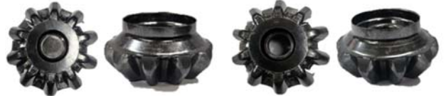
(c) Pinion after forging process (d) Pinion after piercing process
