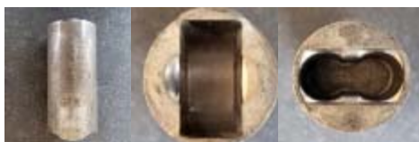
(b) The shape of scorpion body after forming test
