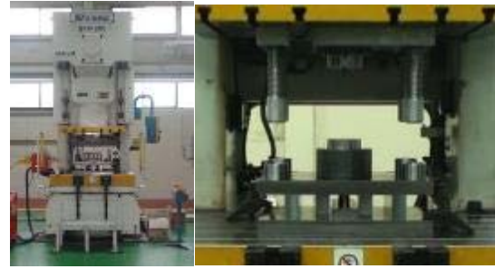
Figure 2: Servo press (SIMPAC) and die set
