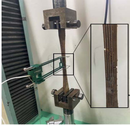
Figure 2: Plywood tensile test jig and photo
