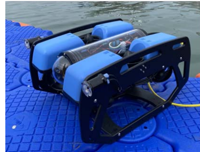
Figure 7: Remotely operated underwater robot used for data acquisition
